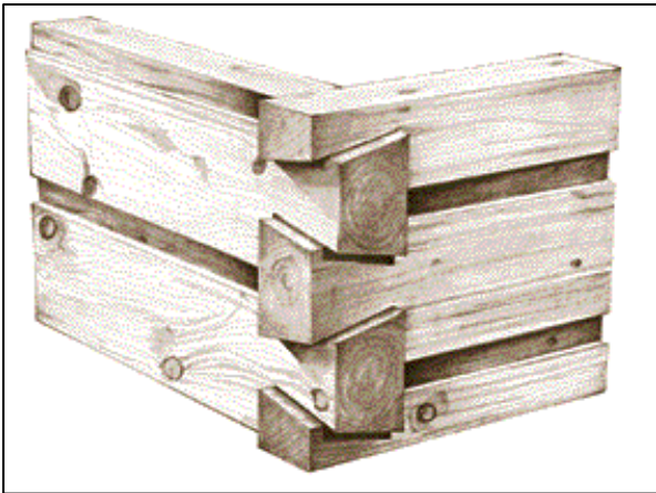
21, 22. Typical dovetail corner joints were used for the connection of wall joists.
